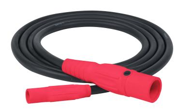
Power Assemblies turn around cable assemblies provide customers a clean, safe and easy way to step up or down cable and connector sizes for portable power applications that use camlock connections. The cables are made from stage cable (Type SC) and the inline camlocks are either Series 16 or Series 15. The turnarounds come in standard lengths of 3, 5, and 10 feet.
